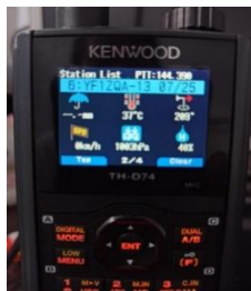
Fig.12. APRS Weather data directly receive on the fly
