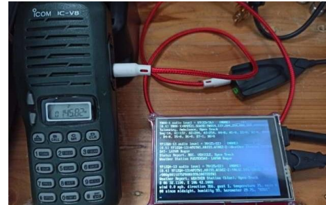
Figure 9. Configuration of data receiver using VHF Radio and Raspberry Pi
