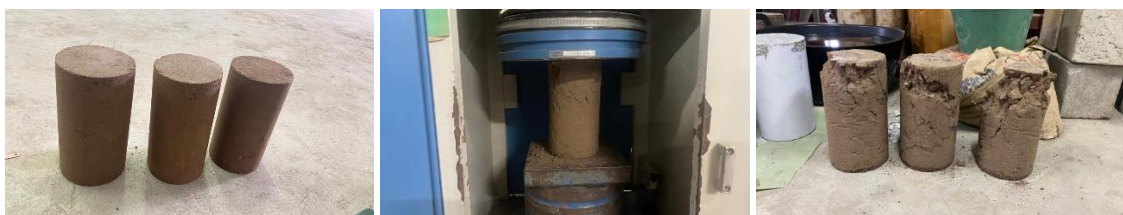
Figure 9. Test results of 10M KOH geopolymer concrete
