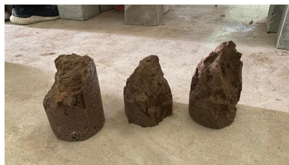
Figure 14. Absorbency test results of 10M KOH geopolymer concrete samples
