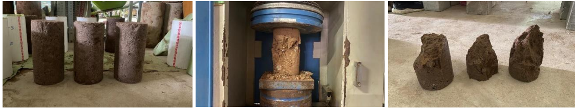
Figure 7. Testing of 8M KOH geopolymer concrete
