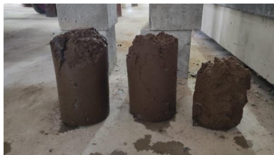
Figure 12. Absorbency test results of 8M KOH geopolymer concrete samples
