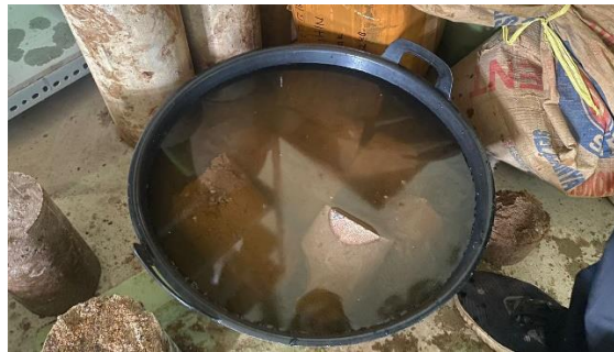
Figure 11. Proses perendaman sampel beton geopolymer
