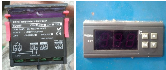
Figure 4. Temperature gauge 220ACV model on engine 3066
