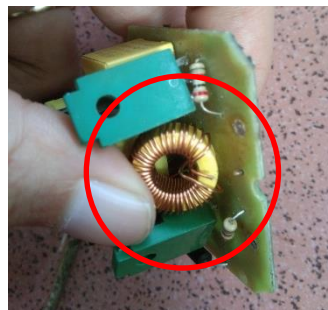
Figure 6. Condition of Step Up Transformer
