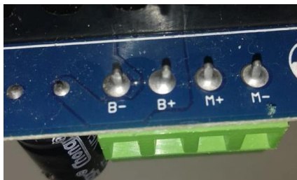
Gambar 7. Pin Output BTS 7960
