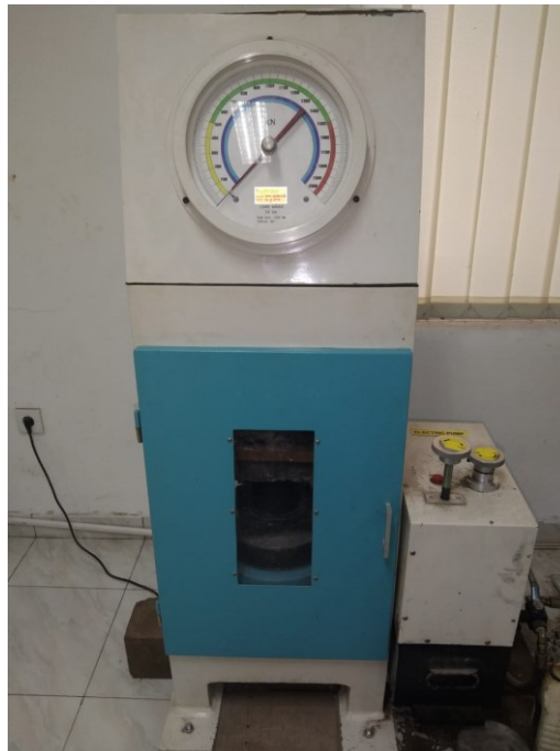
Gambar 2. Mesin uji kuat tekan “Universal Testing Machine.”
