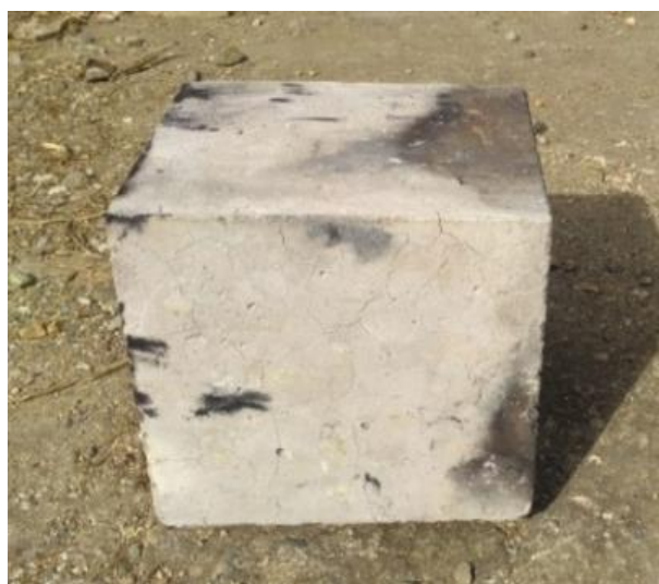
Figure 3. Concrete After Firing Process
