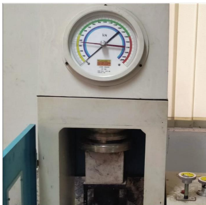
Figure 1. Testing The Compressive Strength of Concrete Samples
