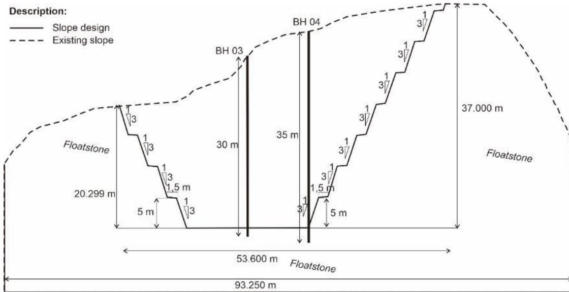
Figure 5. Slope modeling at STA 14+350
