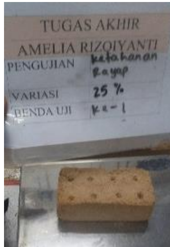
Figure 9. Specimens Condition of Termite Resistance
